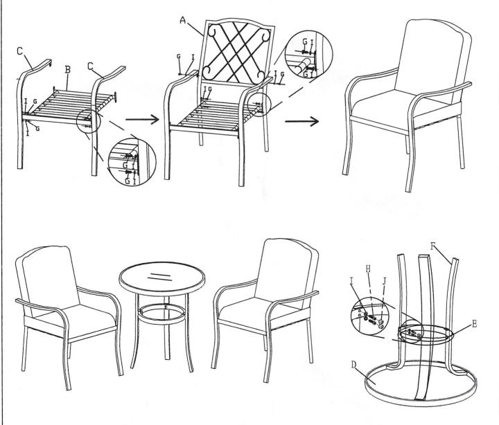
EASY ASSEMBLE TIPS: Tighten each screw about 25% and continue to do so each screw little by little until all screws fully tightened. You might have to pull on the arms and legs a little to align the holes in order for the screws to go in.
